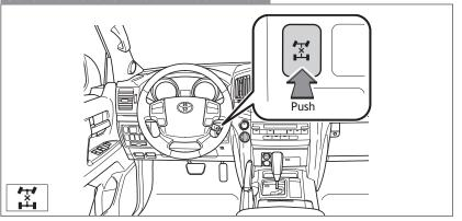
Lock the center differential when your vehicle's wheels get stuck in a ditch or when driving on a slippery or bumpy surface.
